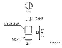
$^{\ast}\text{1:}$  Conversion screw is attached when area code is 3
