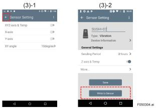
Figure 5-12 Write Adjustment to XS770A
