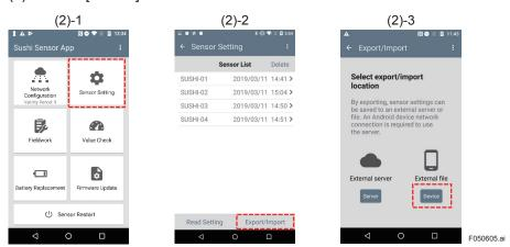
Figure 5-20 Specify Android Device as Import Source
