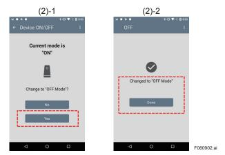
Figure 6-12 Shifting XS770A to OFF Mode
