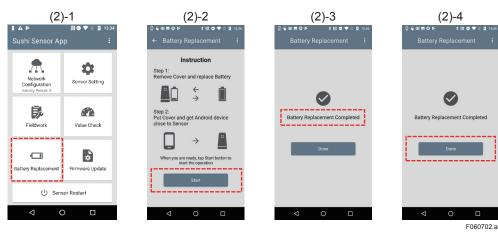
Figure 6-8 Initializing the Battery Life
