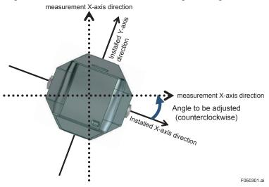
Figure 5-9 Measurement Axis Adjustment
