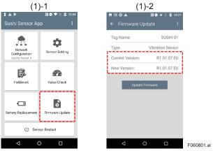
Figure 6-9 Check Current Firmware Version
