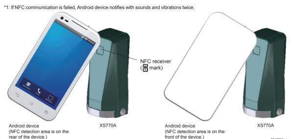
Figure 4-2 The Way of NFC Communication
