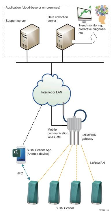
Figure 1-1 Sushi Sensor System Configuration
