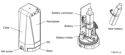
Figure 6-7 Battery Replacement Procedure
