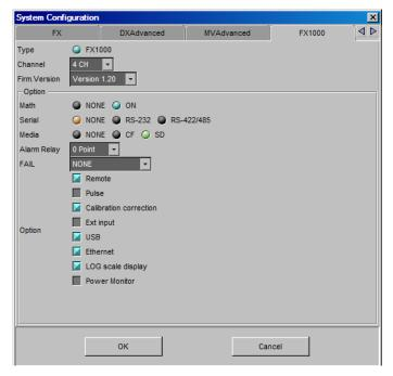
**2.** Change the various settings according to the FX that you will connect to (Blue, orange, and green are used to indicate the selected items. Gray is used to indicate the items that are not selected.).
