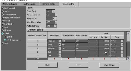
Modbus master settings are enabled when you set [Protocol] to [Master] under [Serial] - [Serial] in the [Basic Setting] tab.
