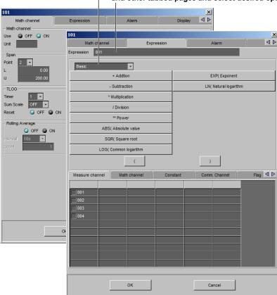
The items in the [Math channel] tab can be configured for each channel. The items that are configured are the same as those configured on the spreadsheet. For details, see the page corresponding to the item.
