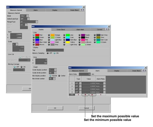
The items in the measurement channel tab can be configured for each channel. The items that are configured are the same as those configured on the spreadsheet. For details, see the page corresponding to the item.
