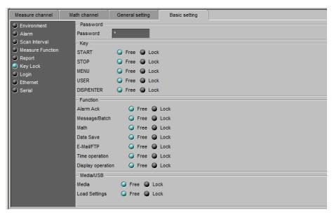
Enabled when [Key Security] is set to [Keylock] under [Environment] - [Detail Setting] in the [Basic Setting] tab.
