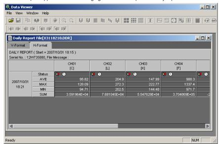
You can select [V-Format] or [H-Format]. The figure above is an example of H-Format. The following figure is an example of V-Format.
