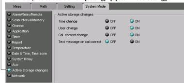
Turn [ON] the setting changes that are allowed when data acquisition is in progress.
