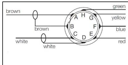
**Figure 10:** Connector layout
