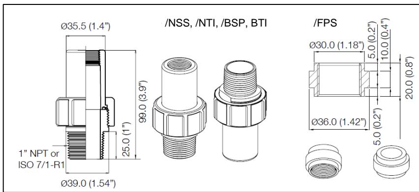
Figure 8: Dimensions 1" FU20-FTS/MTS adapter Stainless Steel & Titanium and FU20 -FTS/MTS adapter for FF40, FS40 and FD40 fittings
