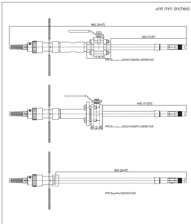
**Figure 5: Dimensional drawing PR10...-D32 with mounted FU20 sensor**
