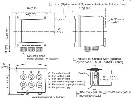
Figure 3.1 Housing dimensions and layout of glands
