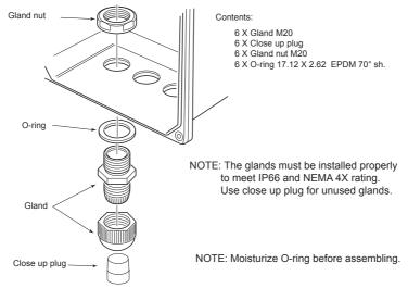
Figure 3.5b How to install cable glands
