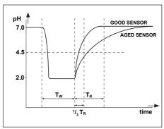
Figure 6.2 Chemical cleaning of sensors
