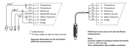
Figure 3.10.b Sensor wiring for combined (pH + Redox) measurement
