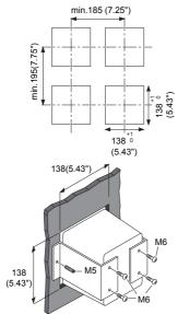
Figure 3.2 Option /PM: panel mounting diagram
