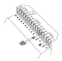
Figure 3.9a. Jumper placement for low impedance setting
