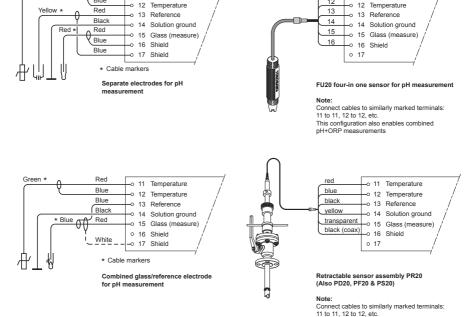
Figure 3.10.a Sensor wiring for pH measurement
