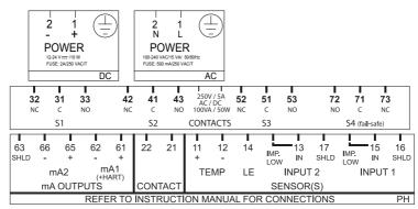
Figure 3.7 Input and output connections
