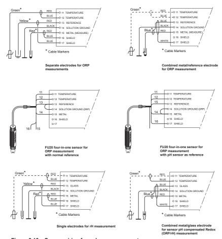
Figure 3.10.c Sensor wiring for redox measurement
