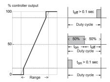
Figure 5.4 Duty cycle control
