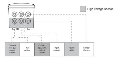
Suitable for cables with an outside diameter between 6 - 12 mm (0.24 - 0.47")
