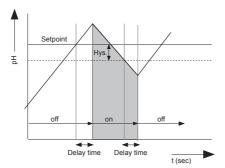
Figure 5.3 Alarm contact (on/off control)
