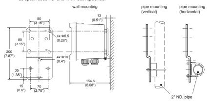
Figure 3.3 Option /U: wall and pipe mounting diagram
