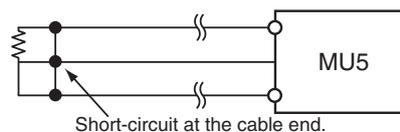
Be sure to turn the adjustment switch counterclockwise to reset the corrected value before executing the wiring resistance correction.
