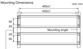
Supplied spacer(50) or Wiring space(30 to 60)
