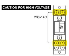
Flexible twisted wire and durable round crimp-on terminal (JIS C2805) are recommended to use
