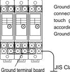
Grounding for serial installation of arresters is to connect ground terminal board in zigzag and touch ground at one point from last arrester according to JIS Class 3 grounding.
