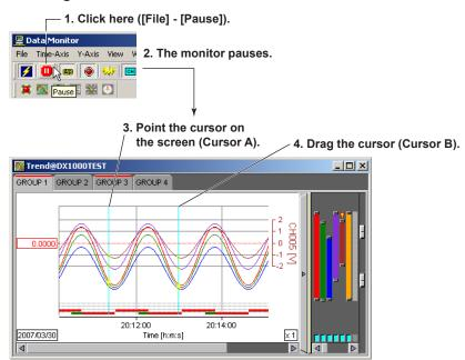
When the mouse is pointed on the screen, Cursor A and Cursor B are overlapped. Cursors can be displayed only when the monitor is paused. Pause the monitor before pointing the cursor on the trend screen.
