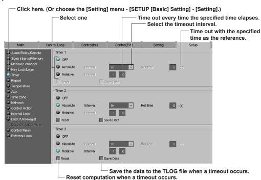
You can set three types of timers to be used in the statistical computation. You can save the data to a TLOG file or reset the computation when the specified timeout interval elapses. This function is available only if the Computation function is installed. For details about the types of timers and various settings, refer to the *CX User's Manual (IM 04L31A01-01E or IM 04L31A01-03E)*.
