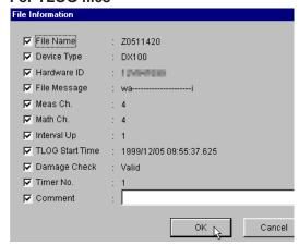
The items that are checked are output in the header when printed.
