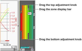
You can change the waveform display zone on the trend display screen by clicking the edit zone icon or by selecting [Y-Axis] - [Edit Zone].
