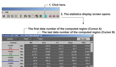
The minimum value, maximum value, P-P, mean, and rms value for each waveform in the range specified by Cursors A and B are computed and displayed. If the cursor is not displayed, the computation is performed over the entire data. If you change a computation condition such as the computation interval and click the [Calculate] button, the results are computed again and displayed.
