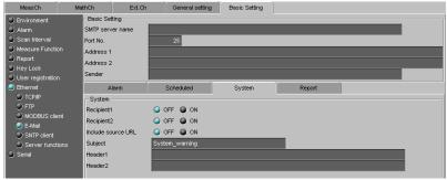
Specify the settings for sending e-mail when the DX recovers from a power failure, at memory end, and when an error occurs.
