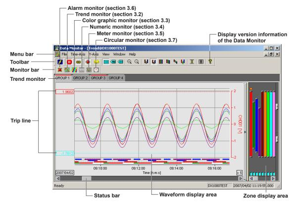
The Data Monitor can be used to monitor the measured/computed data and the alarms of the RECORDER. The following six monitoring methods are available:
