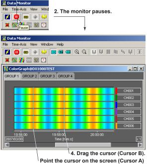
Cursors can be displayed only when the monitor is paused. Pause the monitor before pointing the cursor on the screen.
