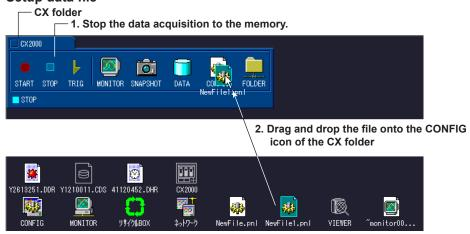
The contents of the setup data file (\*.PNL) located on the DAQ Desktop can be transmitted. If the CX is acquiring data to the memory, the data will not be sent in this case.
