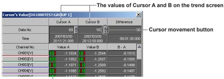
— Alarm display (Displays the conditions of alarm 1, 2, 3, and 4 from the left)
