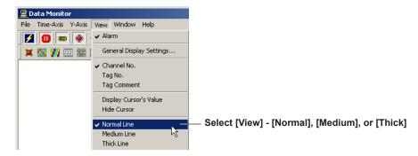
You can select the thickness of the line of the displayed waveform from Normal, Medium, and Thick.
