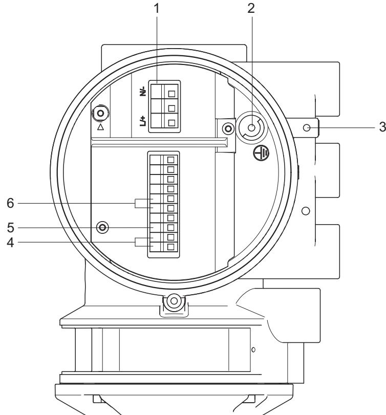
Fig. 7: Terminal box for connection to external devices for Ethernet-APL and for the transmitter power supply
