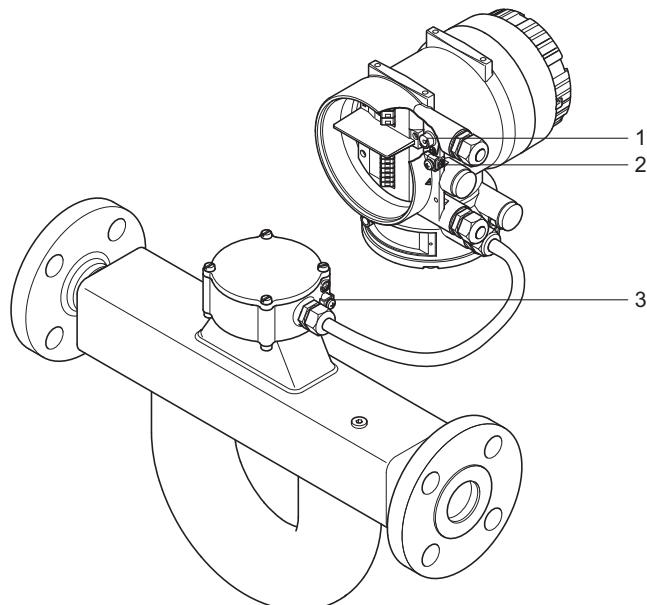
Fig. 3: Grounding connections on transmitter and sensor
