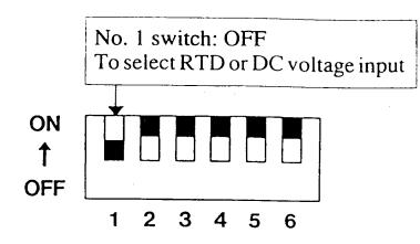
To select RTD or DC voltage input, set DIP switch No. 1 to OFF
