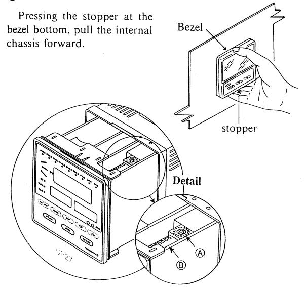
Note: After making the changes, return the internal unit to the case, and turn power ON.
