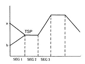
Regardless of the measured value (PV) at program operation start, the program pattern begins with a setpoint equal to the PV and moves linearly toward the target setpoint (TSP) of Segment No. 1.
