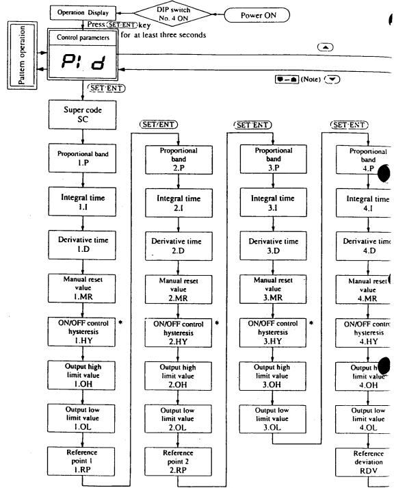
\* If ON/OFF relay output is selected (see p.10), only HY is displayed; P, I, D, MR, OH, OL, RP, and RDV are not displayed.
