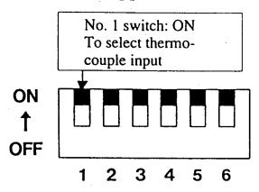
To select thermocouple input, set DIP switch No. 1 to ON
