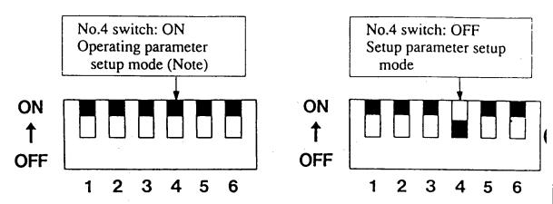
Note: Operating parameter setup mode is called up by pressing the <a href="SET/ENT">(SET/ENT)</a> key for at least three seconds from the Operation Display (see p.22).
