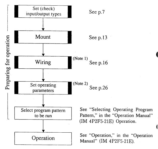
Note 1: The UP27 has no power switch. When power is supplied to it, the UP27 goes to immediately to an operating condition and begins to execute control operations. Therefore we recommend that you not connect its output to the device to be controlled until just before you are ready to begin actual operation.
