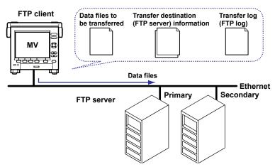
You can specify two destination FTP servers: primary and secondary. If the primary FTP server is down, the file is transferred to the secondary FTP server.
