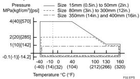
Note 1: This limits show maximum allowable fluid pressure for Flow Tube itself. Further fluid pressure should also be limitted according to flange rating.
