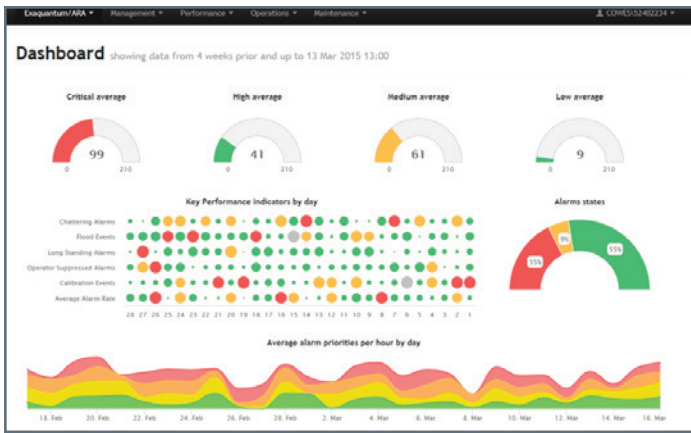
Figure 4: Yokogawa Exaquantum Alarm Reporting and Analysis dashboard is used in a European gas field to summarize activity on 750,000 possible alarms.
