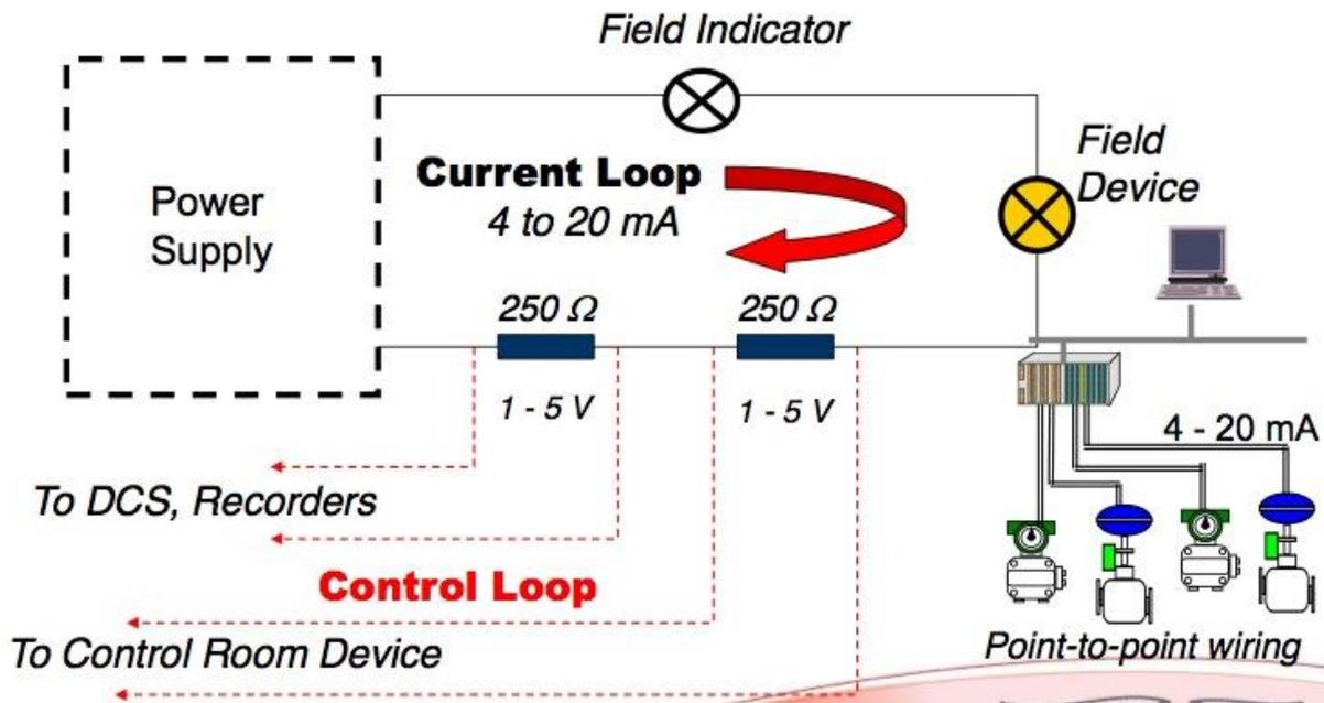
Figure 1. Caption: HART provides a means to access digital data superimposed on existing 4-20mA wiring, making it a low cost fieldbus option.
