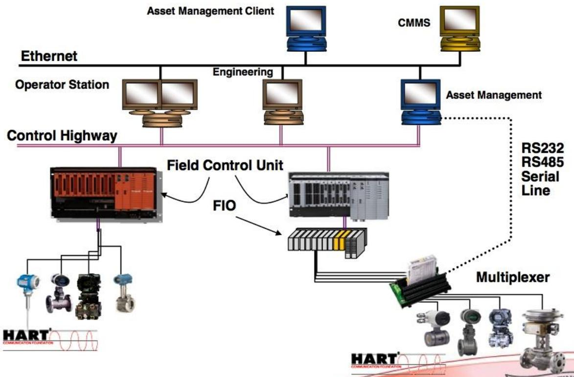
Figure 3. Caption: Native HART-enabled I/O (left field control unit) gathers HART information seamlessly. In systems where HART I/O isn't available, multiplexers can gather information and send it to an asset management system without interfering with the existing I/O flow (right control unit).
