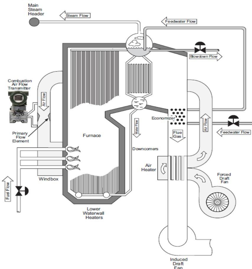
Figure 1: Typical Boiler Combustion Air Flow Measurement
