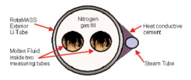
In addition to the external process heating, Yokogawa provides as a standard factory option an insulated enclosure for the RotaMASS sensor:
