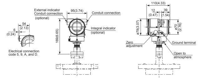
\*1: When electrical connection code 7 or C is selected, a blind plug is protruded up to 8 mm from the conduit connection.
