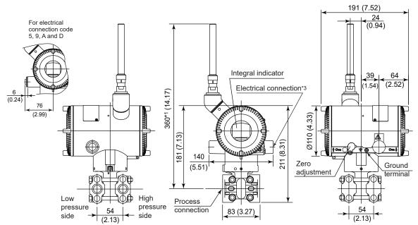
• Wetted Parts Material Code: H, M, T, Measurement Span Code F or Option Code /HD, /HD2
