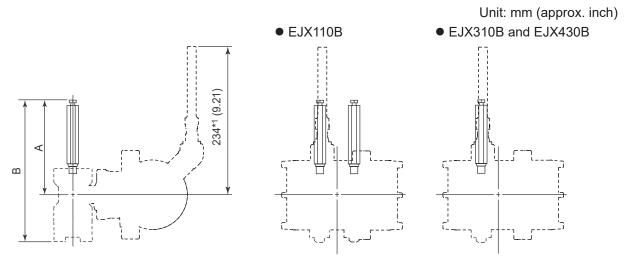
\*1: When amplifier housing code 8 is selected, the value is 234 mm (9.21 inch). When amplifier housing code 9 is selected, the value is 114 mm (4.49 inch). In both cases, the figures are shown as A or B accordingly.
