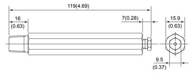
● Long vent plug for oil-prohibited use (when combined with Option code K1, K2, K5, or K6)
