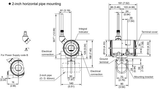
\*1: When amplifier housing code 9 is selected, the value is 187 mm (7.36 inch). In this case, the figure is shown as A.
