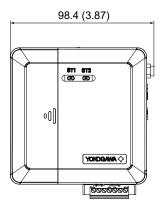
Unless otherwise specified, tolerance is  $\pm 3\%$  (however, tolerance is  $\pm 0.3$  mm when below 10 mm).
