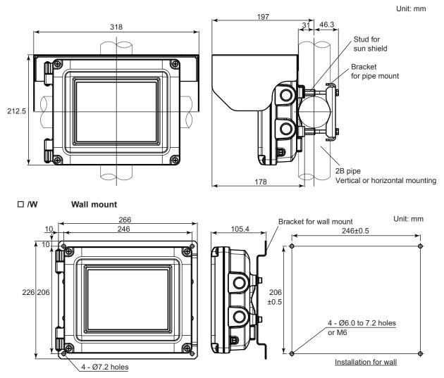
\*: The wall construction for mounting has to be designed for 4 times the weight of the YH8000. Bracket for wall mount can be placed in lengthwise
