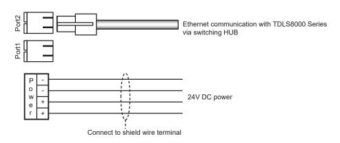
• Maximum cable length between YH8000 and Switching HUB is 100m.
