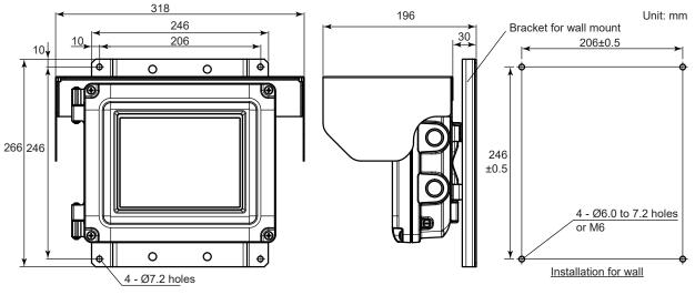
\*: The wall construction for mounting has to be designed for 4 times the weight of the YH8000. When the sun shield is mounted, the bracket for wall have to be placed in widthwise. Unless otherwise specified, differences in the dimensions are specified as: General tolerance = ±(Criteria of tolerance class IT18 in JIS B0401-1998)/2.
