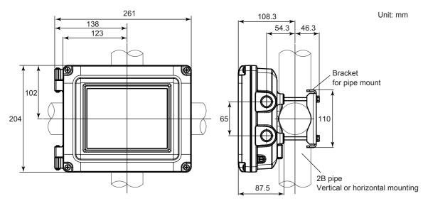
Unless otherwise specified, differences in the dimensions are specified as: General tolerance = ±(Criteria of tolerance class IT18 in JIS B0401-1998)/2.
