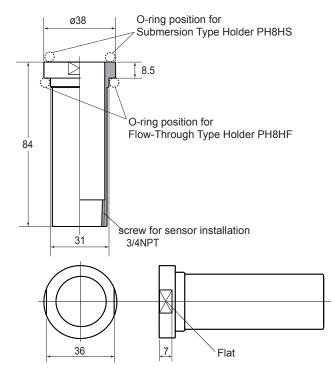
Unless otherwise specified, differences in the dimensions are specified as: General tolerance = ±(Criteria of tolerance class IT18 in JIS B0401-1998)/2.
