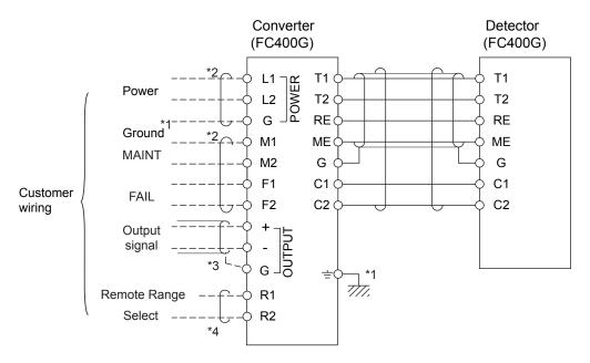
(Note) All are connected to wiring terminals (M3 screw) in the converter.
