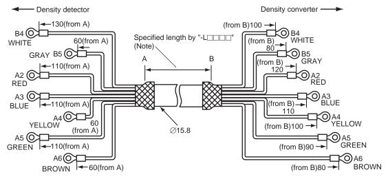
(Note) Cable length is specified by the suffix code of "-L $\square$ " ,  $\square$  is specified in meter. e.g. for 50 m, -L0050 for 100 m, -L0100 for 2 km, -L2000
