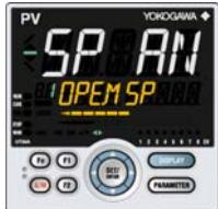
3. Press the SET/ENTER key to display the [SP] Parameter Setting Display.
