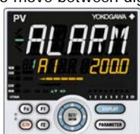
7. Press the SET/ENTER key to register the setpoint (the setpoint stops blinking).
