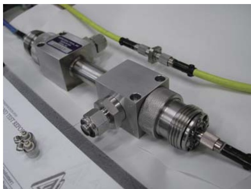
Figure 2.21 FT-NIR Gas measurement cell
