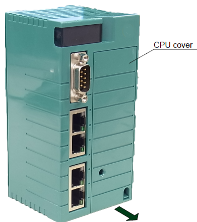
Figure Removing CPU Cover
