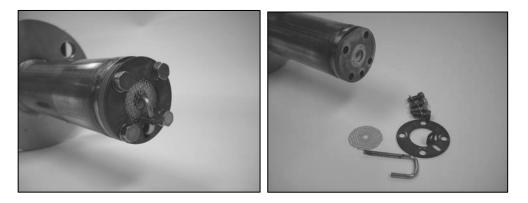
2. Remove the Zirconia cell and metal o-ring. Ensure that when removing the Zirconia cell, it is rotated in the direction etched on the face of the cell. (Should be clockwise). Failure to do so may damage the contact spring.
