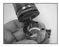
5. Apply anti-seize compound to the bolt threads. Insert the bolts, and torque to 51 in/lbs.
