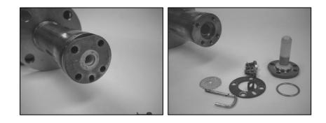
3. Do not re-use the metal o-ring. The dust and oil filter comes with a new metal o-ring that should be used. Replace Zirconia cell (ensuring that the cell is rotated clockwise as it is inserted), plate, calibration tube, and filter screen.
