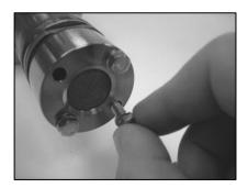
The E7042UQ Dust and Oil Filter installation is now complete, and the ZR22 Oxygen Probe can be installed.
