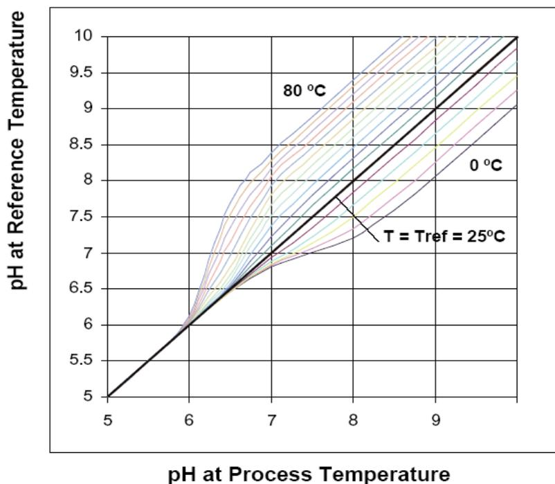
For pure makeup water or boiling water reactor samples, the solution temperature coefficient should be set to  $-0.016 \text{ pH}/^\circ\text{C}$ . For ammonia, phosphate and/or amine-treated water, the solution temperature coefficient should be set to  $-0.033 \text{ pH}/^\circ\text{C}$ . For other process solutions the correct solution temperature coefficient can be calculated by developing temperature vs. pH data. The negative slope of this data is the solution temperature compensation value.
