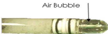
Why is the air bubble an issue? The inner gel layer under the air bubble dries out. When placed into service in a normal upright position the inner gel layer will recover. Many end users will do a second calibration after 24 hours of run time to correct for the inner gel layer’s recovery.
