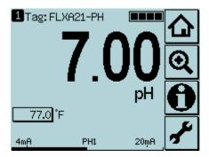
Previously you should have calculated what the Solution Temperature Compensation value is for you Process Solution. Enter that value of the keypad.
