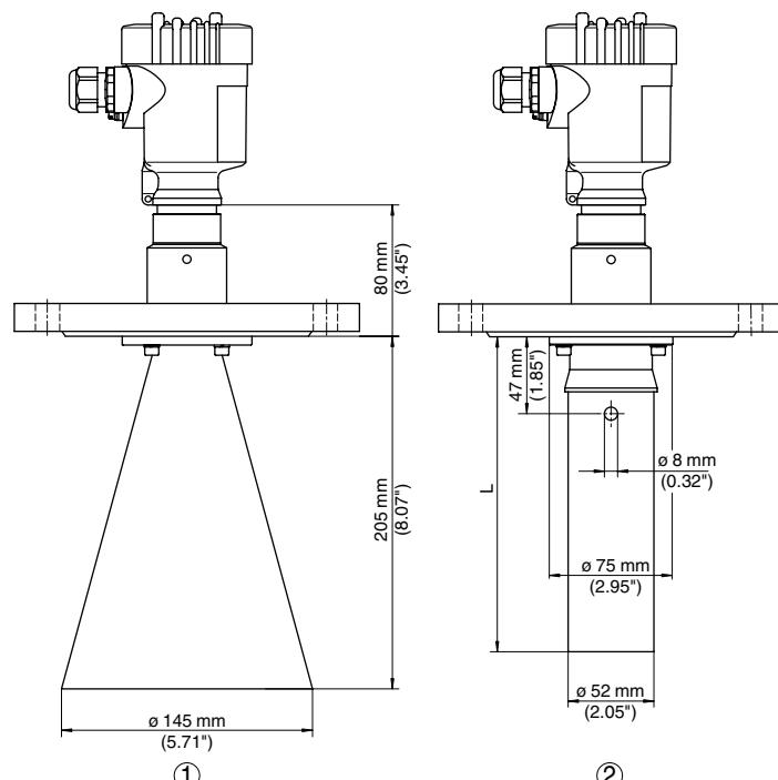
1 Version with horn antenna  $\varnothing$  145 mm
