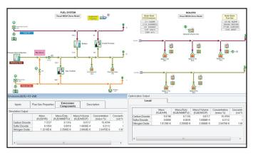
EP-RTO chooses the most economic fuel to burn in the boilers and/or process heaters. The fuel system can be modeled in great depth to include emissions limits, CO<sub>2</sub> trading and contractual issues, such as fuel oil grades, natural gas suppliers, quotas and penalties if the former are exceeded. When cogeneration options are available the fuel/steam tradeoff can yield economic benefits.
