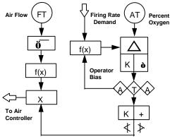
The output of the percent oxygen controller is adjusted for gain and bias and applied to the combustion air flow signal. Additionally, low and high limits are used to ensure continued operation during analyzer outage.
