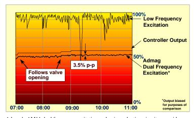
Admag's AM11 dual frequency excitation and noise reduction circuitry provides a more stable output than can be obtained with low frequency, pulsed DC systems.
