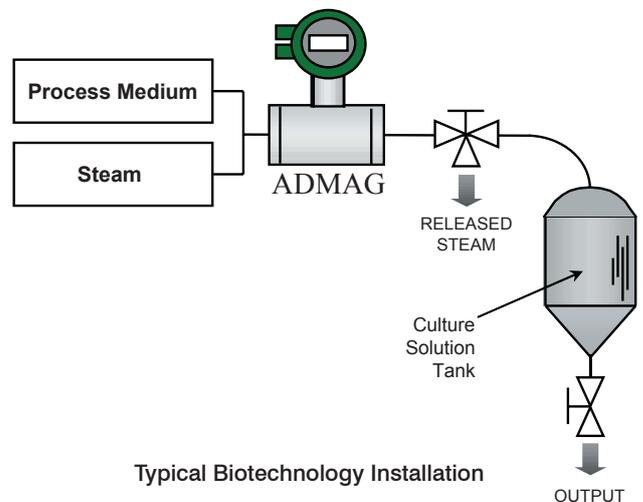
Place) applications can subject meters to drastic temperature fluctuations in short periods of time. These temperature swings can lead to a variety of failures in meters with inferior design and materials of construction. Electrode seals can fail due to differing expansion rates of the liner and electrodes, and inferior liner materials can crack and fail, causing leakage or loss of the measurement.
