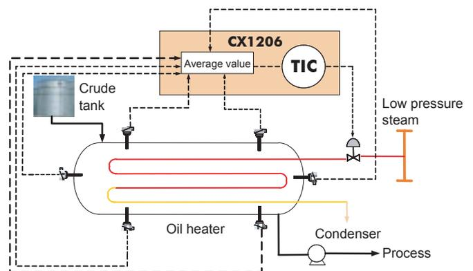
The process shown in the example above formerly required six temperature converters, three computing units, and one controller (ten units in all), but the CX integrates all of these into a single unit for a less expensive, more reliable solution.
