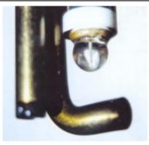
These two pictures show identical sensors installed on the same application for the same time duration. One sensor has on line cleaning applied and is in excellent condition with many years life still remaining. The other has not been cleaned, it has a high reference resistance, slow response and will soon be unserviceable.
