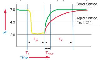
Another maintenance saving feature is the transmitters ability to cope with changing measurement conditions. For example if the coating nature of the water increases for any reason (e.g. oil in waste water), then the impedance diagnostic can be used to internally trigger the wash system independent of the normal timing. This means that transient effects are compensated within the instrument without generating any external alarms thereby saving unnecessary call outs.
