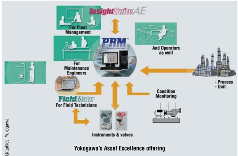
their make or field communication protocol. FieldMate speeds up device configuration and problem solving, and automatically stores a work log for a traceable field maintenance database that consolidates the maintenance work flow and facilitates the sharing of maintenance know-how.
