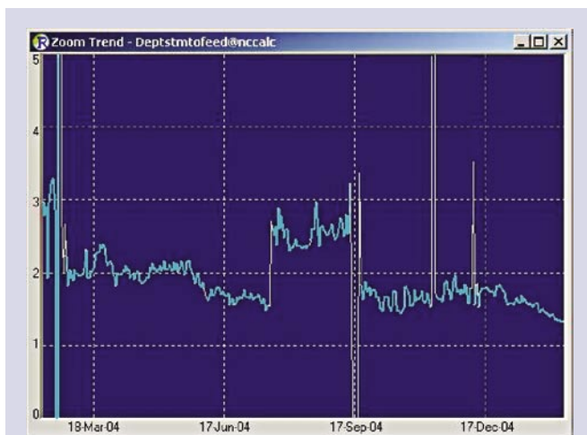
FIG. 3 Starting Dec. 17, the depentanizer steam-to-feed ratio started dropping and showed much improved stability.
