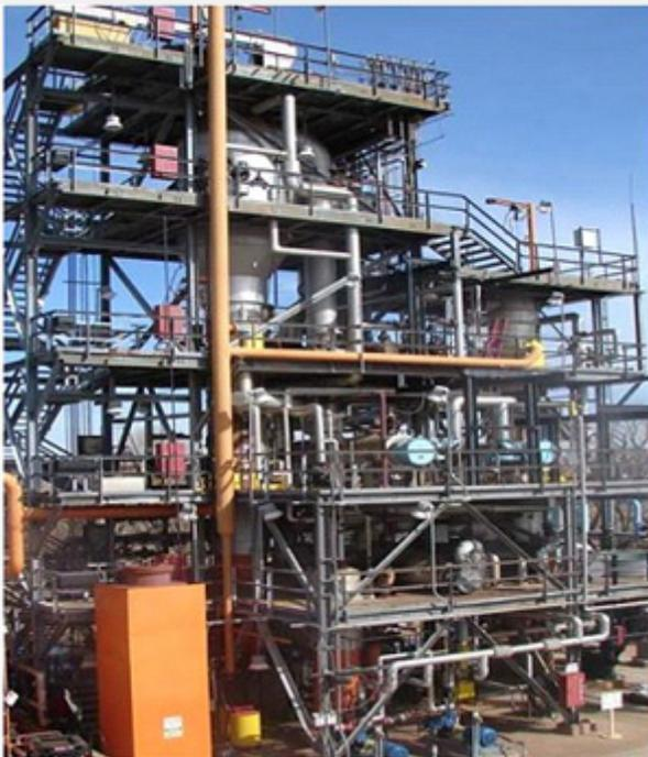
Figure 1: These columns are used by FRI to test and study distillation on behalf of member companies.
