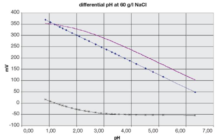
In this graph we see that the sensor is only linear down to 3 pH and the Isopotential value is now 8 pH or the Asymmetry Potential at 7 pH is + 60 mV.
