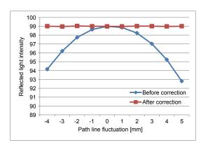
Figure 8 Comparison of the reflected light intensity before and after the correction
