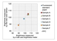
Figure 2 Comparison between the measurement results of the new color sensor and those of a laboratory-use brightness meter (ISO Brightness)
