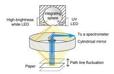
Figure 3 Conceptual diagram of the optical system
