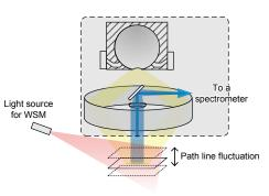
Figure 5 Structure for the WSM
