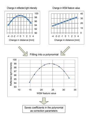
Figure 7 Determining correction coefficients used for the WSM
