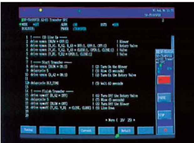
Figure 5 Example of SEBOL Program for TRANSFER
