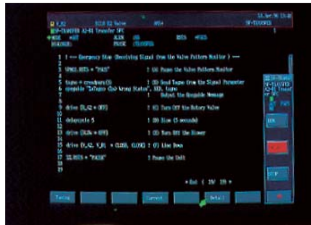
Figure 6 Example of SEBOL Program for EMSTOP
