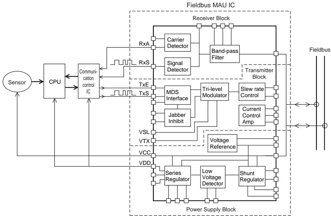
**Figure 1** Block Diagram of Fieldbus MAU IC and an Example of External Connection
