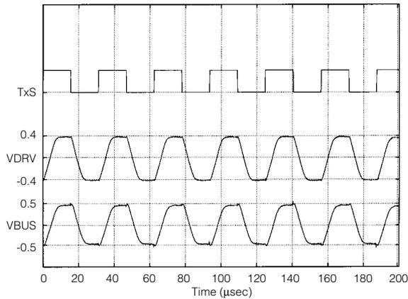
**Figure 6** Signal Waveforms at Transmitter Block
