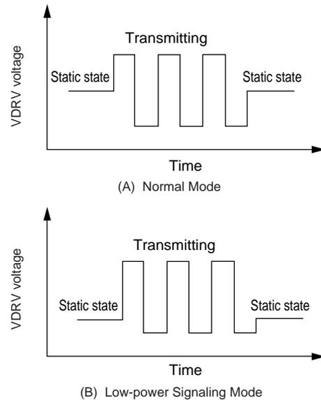
**Figure 3** Waveforms at VDRV Terminal
