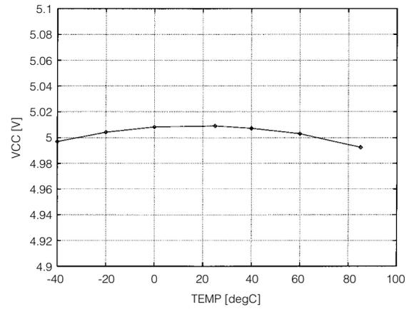
**Figure 5** Shunt Regulator's Output Voltage vs. Temperature
