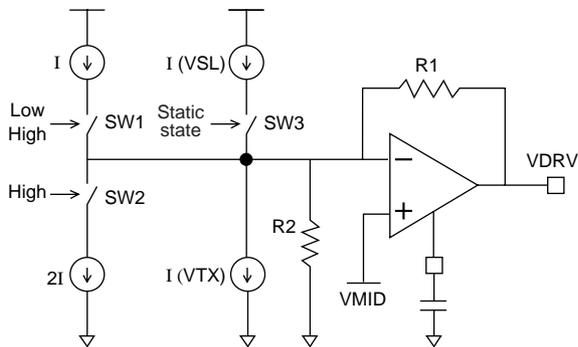
**Figure 2** Circuit Diagram of Connected Tri-level Modulator and Slew Rate Control Circuit
