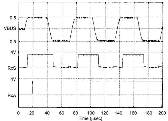
**Figure 7** Signal Waveforms at Receiver Block
