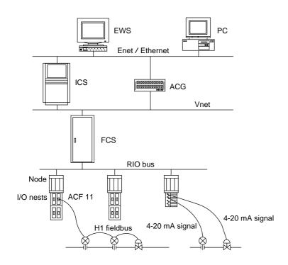
Figure 1 CENTUM CS System Configuration
