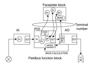
Figure 4 Operation and Monitoring Using a Faceplate Block
