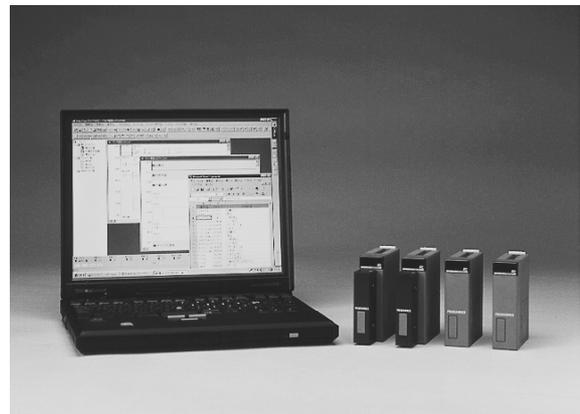
**Figure 1** CPU modules of FA-M3 R and Windows of WideField
